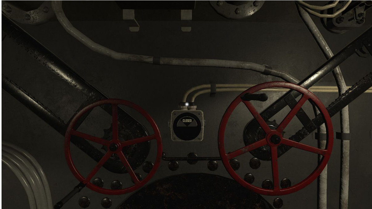
The ballast vents are located in the front and back of the control room.
